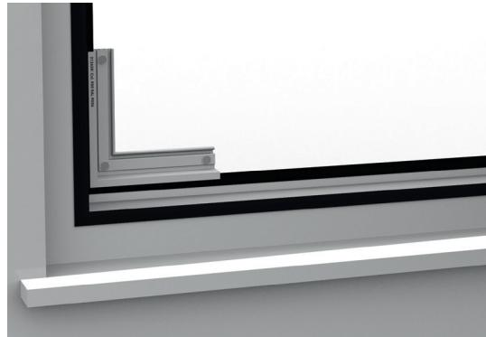
Place angle into the left bottom corner of the external window frame. Close the window.
