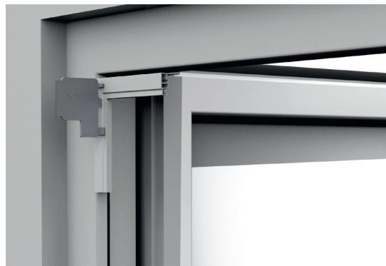
Hold angle in the left/right corner of the external window frame and check how much room is needed.
